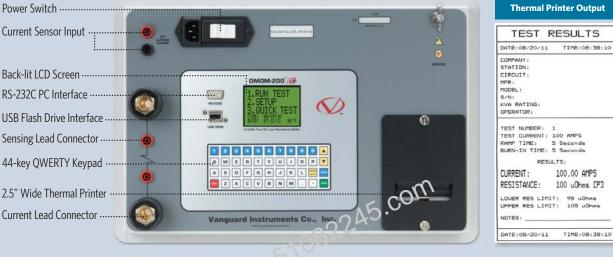
Built-in Thermal Princet P thermal printer that can be used to print test reports in the field.
