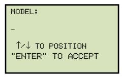
Type the transformer's model information using the alpha-numeric keypad and then press the [ENTER] key.
