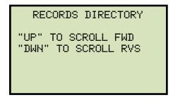
Press the **[Contrast**  $\land$ **]** or **[Contrast**  $\lor$ **]** key to scroll through the test record directory. The test record header will be displayed as shown:
