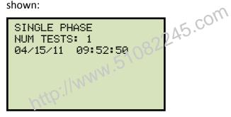
Press the **[Contrast** ∨] key. The test record details will be displayed as shown:
