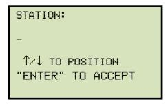
.. and t. N.51082245.COM Type the station name using the alpha-numeric keypad and then press the **[ENTER]** key.
