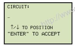
Type the circuit information using the alpha-numeric keypad and then press the [ENTER] key.
