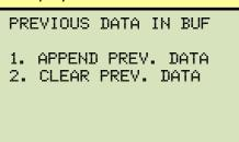
Press the **[1]** key (*APPEND PREV. DATA*) to append the data in the unit's working memory to the current test results, or press the **[2]** key (*CLEAR PREV. DATA*) to clear any previous data from the unit's memory buffer and only save the current test results.
