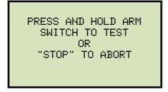
Press and hold the [ARM] switch to initiate the test.
