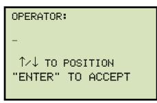
Type the operator's name using the alpha-numeric keypad and then press the **[ENTER]** key. All header information will be saved, and you will be returned to the "START-UP" menu.
