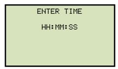
Enter the current time using the alpha-numeric keypad. When the complete time has been entered, you will be immediately returned to the "START-UP" menu.
