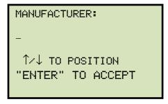
Type the manufacturer name using the alpha-numeric keypad and then press the [ENTER] key.
