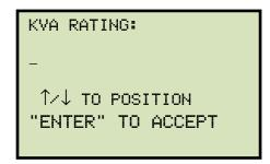
Type the transformer's KVA rating using the alpha-numeric keypad and then press the [ENTER] key.
