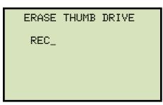
Type the record number that you would like to erase using the alpha-numeric keypad and then press the **[ENTER]** key. The test record will be erased from the USB Flash drive and the following screen will be displayed:
