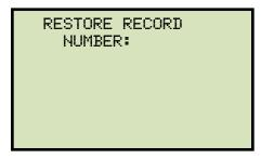
Type the record number using the alpha-numeric keypad and then press the **[ENTER]** key.
