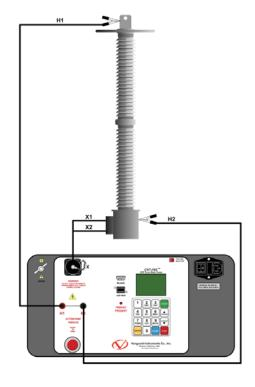
The CVi-765 can measure the turns-ratios of Capacitor Voltage Transformers ranging from 75 to 15,000. The measured turns-ratio, winding polarity, and winding phase angle are displayed on the unit's LCD screen.
