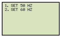
Select the preferred frequency by pressing the corresponding key on the keypad ([1] or [2]). The frequency will be set and a confirmation screen will be displayed as shown below:
