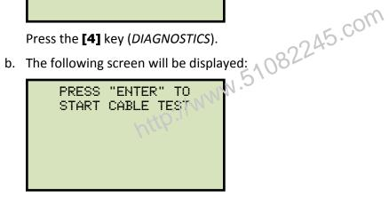
Open the breaker and then press the **[ENTER]** key.
