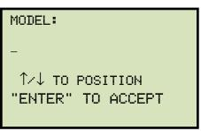
Type the circuit breaker's model information using the keypad and then press the [ENTER] key.
