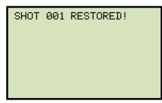
The test shot will be restored to the unit's working memory. You can then view or print the test shot information using the instructions in section 3.6.1.
