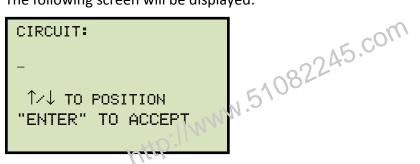
Type the circuit information using the keypad and then press the **[ENTER]** key.
