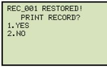
Press the **[1]** key (*YES*) if you would like to print the test record, or press the **[2]** key (*NO*) if you do not want to print the test record. The test record will be restored to the unit's working memory, and you will be returned to the "START-UP" menu.
