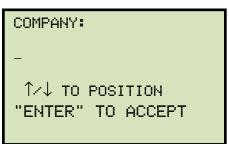
Type the company name using the keypad. Press the **[ENTER]** key when you are done typing the company name.
