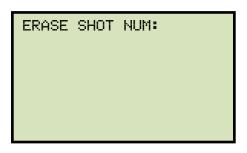
Type the record number that you would like to erase using the keypad and then press the [ENTER] key. If you do not know the test record number, you can first print the test record directory using the instructions in section 3.6.6.
