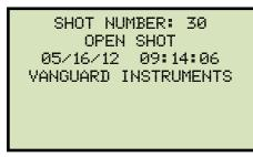
When you have located the test record that you would like to restore, press the **[ENTER]** key. The test shot will be restored to the unit's working memory. You can then view or print the test shot information using the instructions in section 3.6.1.
