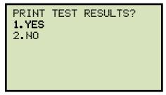
Press the [1] key (YES) to print the test results on the unit's built-in thermal printer.
