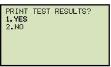
Press the [1] key (YES) to print the test results on the unit's built-in thermal printer.
