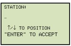
Type the station name using the keypad and then press the **[ENTER]** key.
